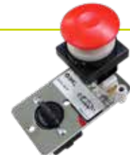
SAI4-2108 - 3/2 NC/NO valve, operated by a knob
